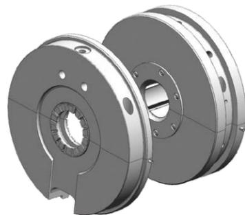
Independent thrust and journal bearings enhance mechanical reliability for a wide range of loads and eliminate hot oil carryover, reducing bearing pad temperatures. Thrust bearing designed to limit axial rotor float, enabling high stage efficiency.
